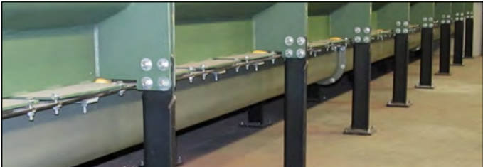
Screw Conveyor System: Assembled in sections for various trap widths and easy maintenance access.
