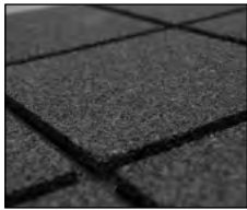
Crumb Rubber: High splatter absorption, low sound reduction.
