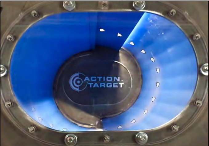
9mm bullet decelerating inside Vortex test chamber (white path).
