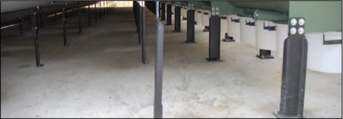
Trap Legs: Flat floors are often uneven. Adjustable height legs ensure that the trap stays level on any floor.
